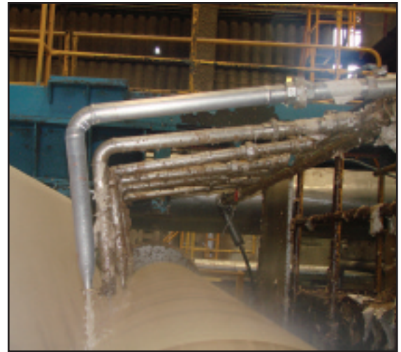
(Above): The foremost pipe is covered in a .020" thick FEP sleeve. Note the difference in build up between the FEP-covered pipe and the uncoated pipes.
