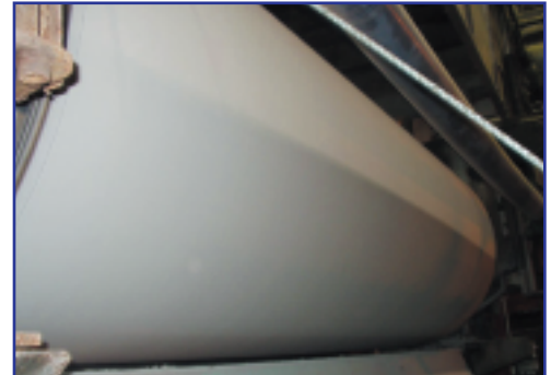
Fluoro-Coat™ 200 is often applied to dryers immediately after press sections.
