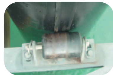
Roll covers are made with a butt seam. In this application it was desirable to have a cap-strip to provide additional wear resistance at the bearing points.
