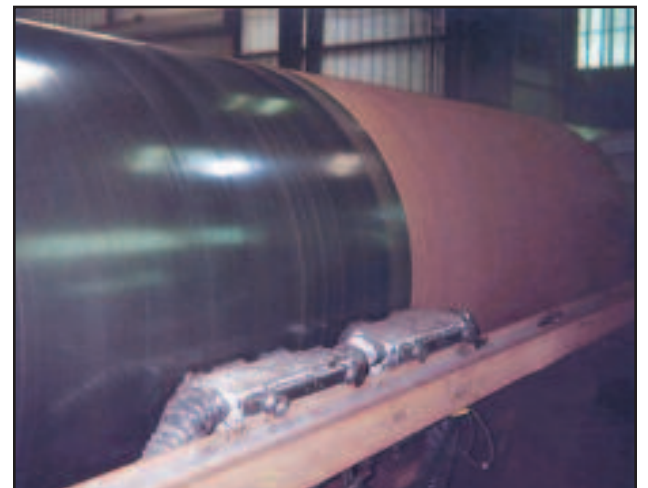
First pass with Fluoron's BCS Roll Cleaning System
