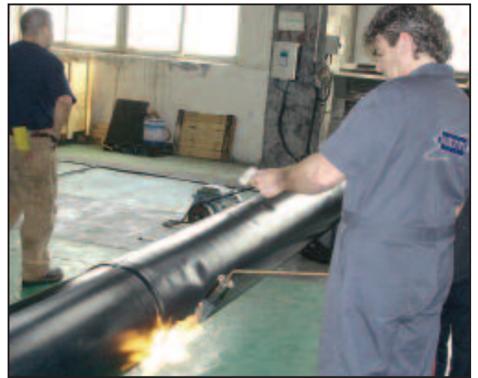
This roll cover installation was completed in 3 hours in the paper mill's aisle.
